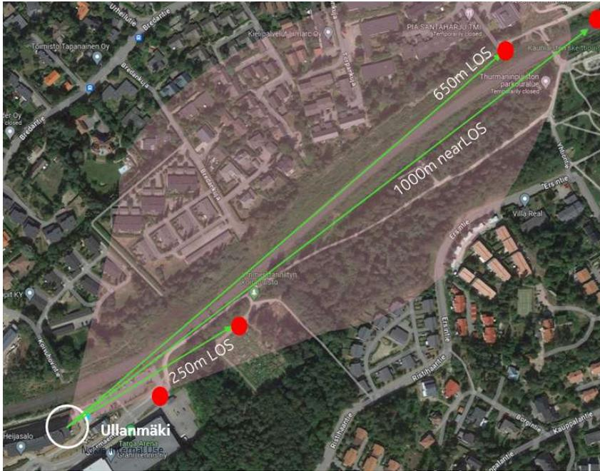
Initial findings: Based on outdoor-to-outdoor field measurements, the RSRP<sup>5</sup> values (UL coverage) for 7GHz are equal to 3.5 GHz up to a 650 m distance from the rooftop antenna. Above this distance, the RSRP value attenuates more for 7 GHz as compared to the 3.5 GHz spectrum: 9 dBm attenuation at 790 m away from the antenna, and 12 dBm respectively, when 1000 m away from the radio. Nokia will publish more measurements during Q4 2024.
