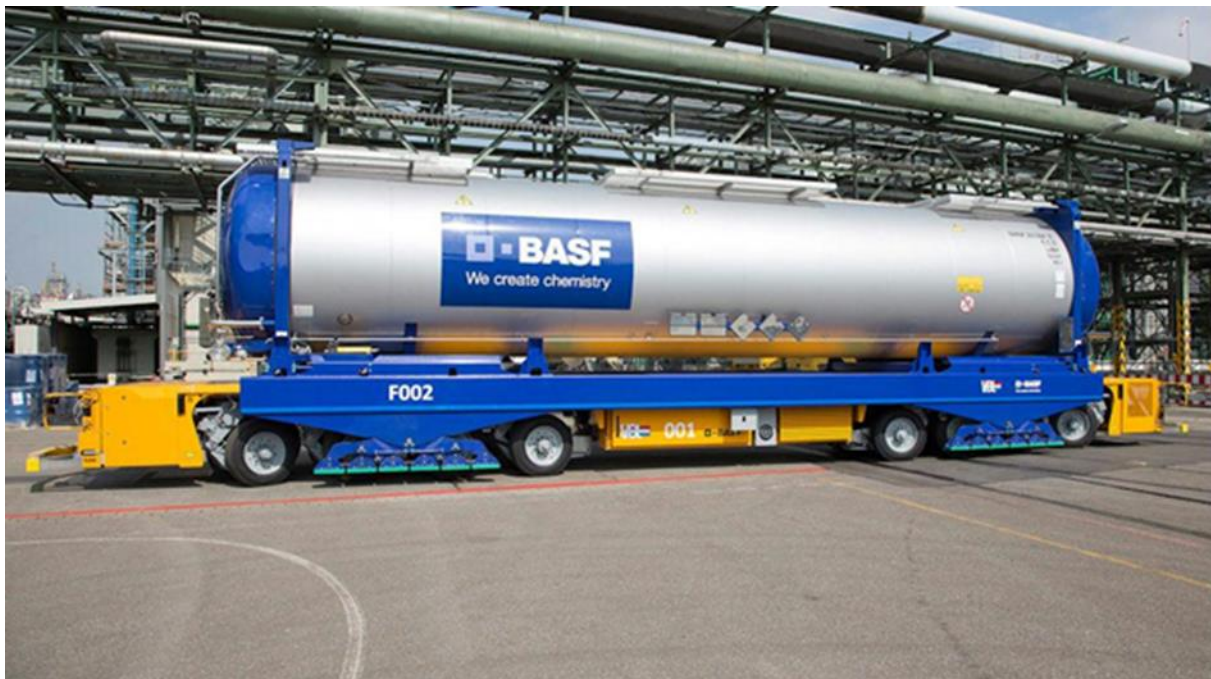
Figure 4: Fully automatic conveyor vehicle
